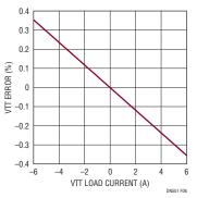
Figure 6. VTT Load Regulation (Figure 2 Design)
