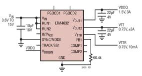
Figure 1. Typical LTM4632 DDR3 Application
