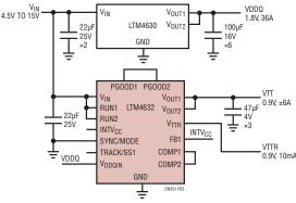
Figure 2. LTM4632 Two Phase Single Output ±6A VTT with 36A LTM4630 VDDQ Supply
